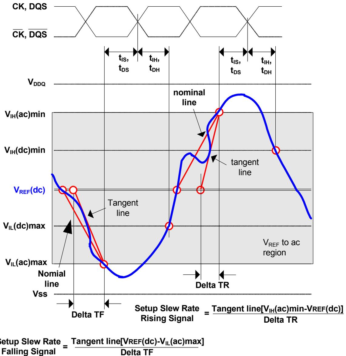
**Fig. c. Illustration of nominal line for  $t_{IH}$ ,  $t_{DH}$**
