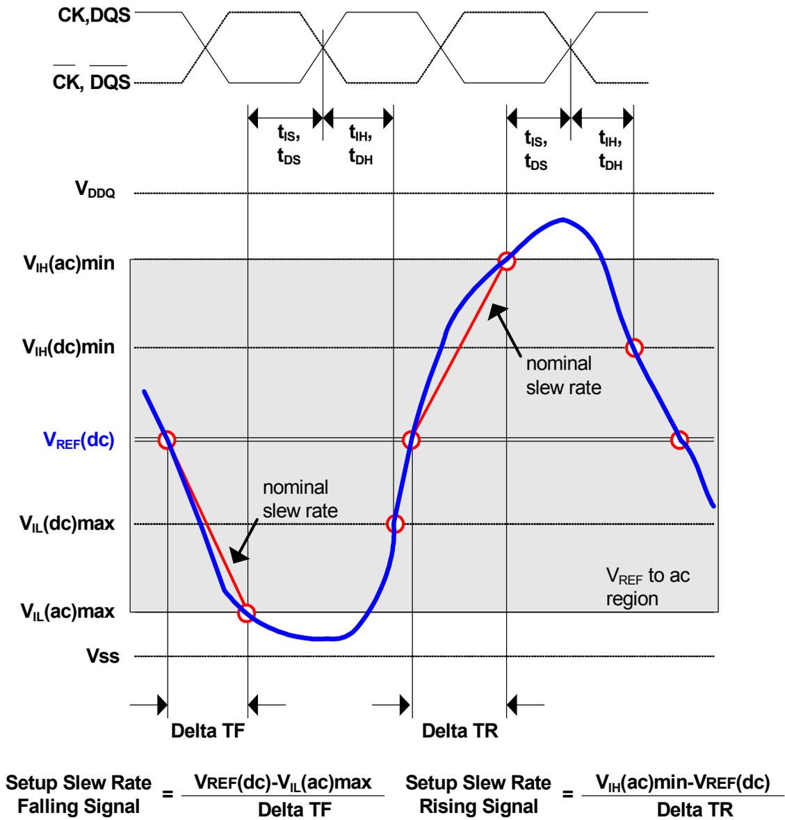
Fig. b. Illustration of tangent line for t<sub>IS</sub>,t<sub>DS</sub>
