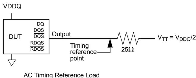
The output timing reference voltage level for single ended signals is the crosspoint with V<sub>TT</sub>. The output timing reference voltage level for differential signals is the crosspoint of the true (e.g. DQS) and the complement (e.g.  $\overline{DQS}$ ) signal.
