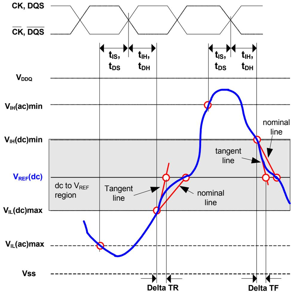
$$\text{Hold Slew Rate Rising Signal} = \frac{\text{Tangent line}[V_{REF}(dc) - V_{IL}(ac)max]}{\text{Delta TR}}$$
