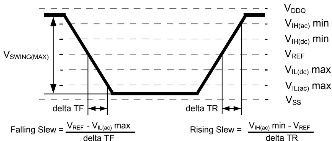
edges and the range from  $V_{REF}$  to  $V_{IL(ac)}$  max for falling edges as shown in the figure below.
