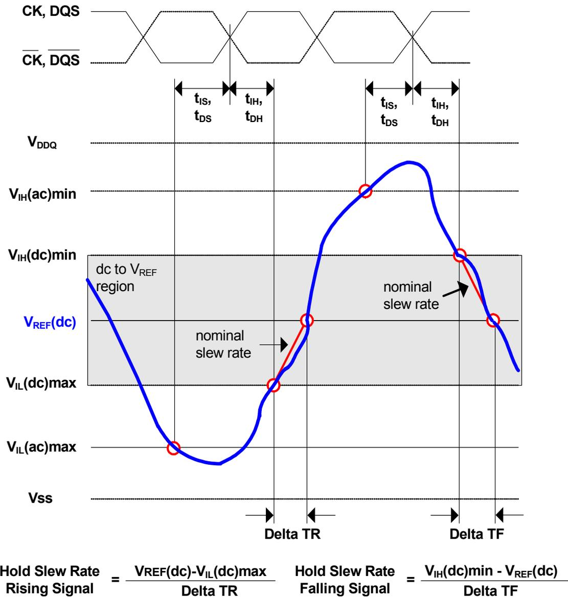
**Fig. d. Illustration of tangent line for t<sub>IH</sub>, t<sub>DH</sub>**
